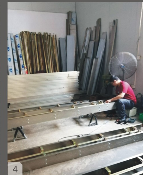
4 尾架组装 Conveyor assembly
