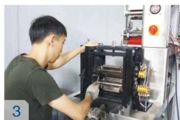
3 刀座调试 Sealing cutter jaw debugging
