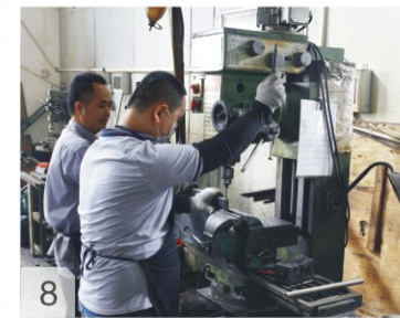
8 钻孔攻牙 Drilling and tapping
